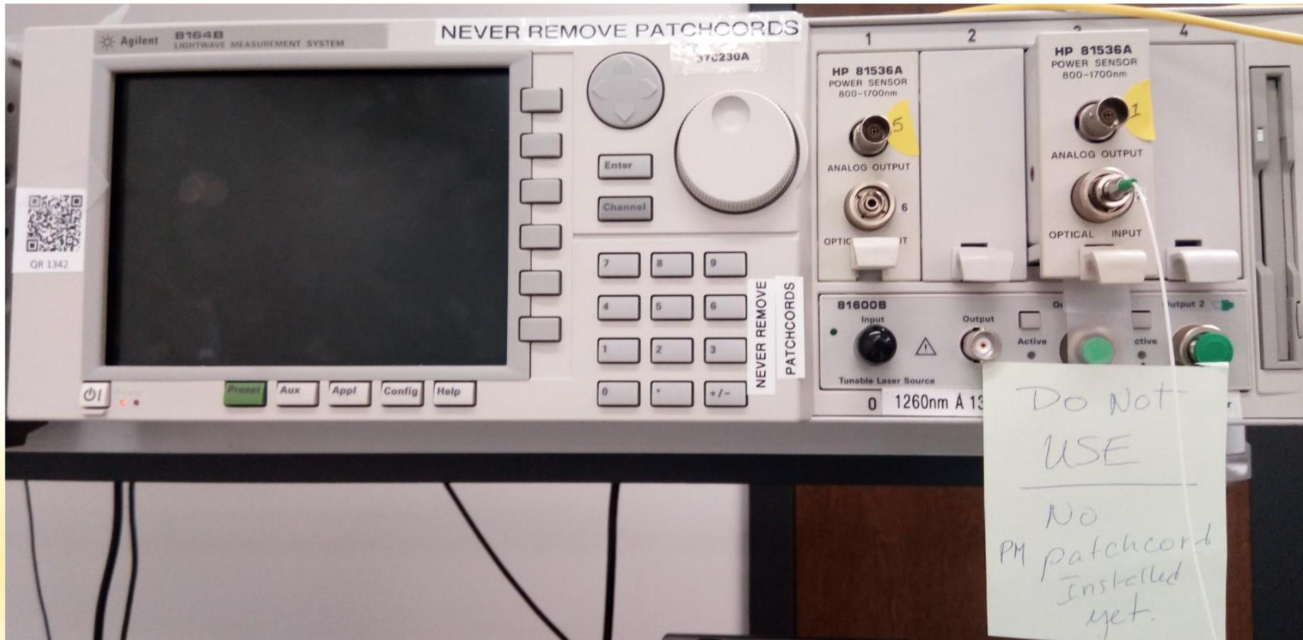
A new PM fiber has to be added as connector saver to the laser module, at the bottom right.
