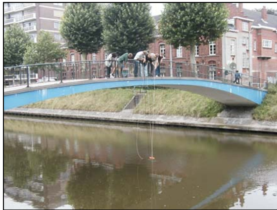
Figure 4.12 Deployment of ADCP in channel Coupure, located in Ghent (Belgium)
