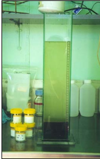
Figure 5.3 Rectangular sedimentation column
