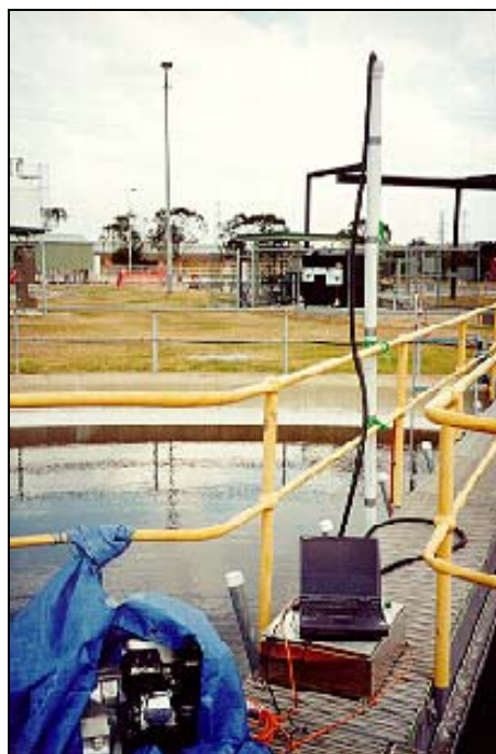
Figure 6.1 Experimental layout for in situ particle sizing
