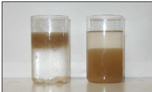
Figure 1.2 Example of rising sludge (left) as compared to normal settleable sludge (right)
